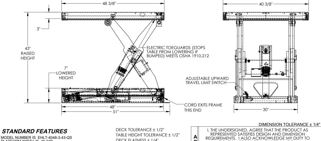
PLATFORM WIDTH IS 40 3/8" PLATFORM LENGTH IS 48 3/8" **OVERALL LENGTH IS 51"** PLATFORM RAISED HEIGHT IS 43" PLATFORM LOWERED HEIGHT IS 7" TABLE CAPACITY (EVENLY DISTRIBUTED) LOAD IS 3.000 LBS CONTROL IS HANDHELD, 2 BUTTON, NEMA 4 PENDANT WITH MINIMUM 8' USABLE COIL CORD SAFETY MAINTENANCE PROPS, DISPLACEMENT STYLE CYLINDERS INSTALLED ROD DOWN EMERGENCY SAFETY STOP HYDRAULIC FUSES IN ALL CYLINDER UNITS HAVE 2' TEST LEAD AND PIG TAIL DURABLE LIQUID PAINT BLUE FINISH INTERNAL POWER UNIT
